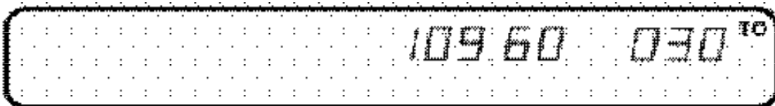
VOR MODE: ACTIVE "BEARING TO" FUNCTION DISPLAY
