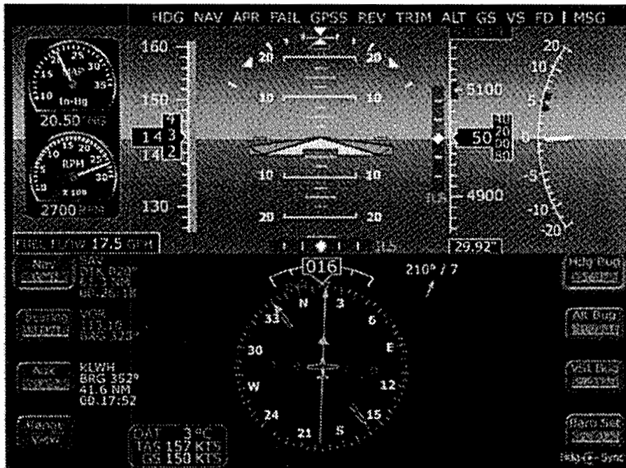
Figure 1 - Entegra 700-00006-0XX-( ) Primary Flight Display
